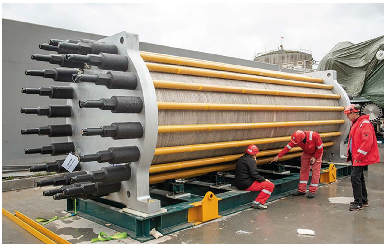
Fig 2: Large electrolyser tested by HydrogenPro in Q4 2022 5
